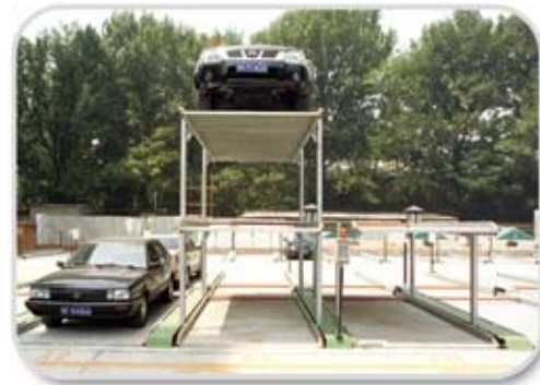
北京园景花园 PJS-3简易升降式 132车位 Beijing Yuanjing Park Apartment PJS-3 Mini parking system—having 132 parking seats
