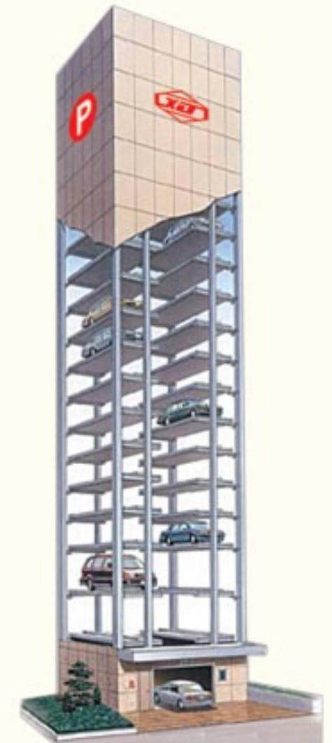
PCS Vertical Lifting Mechanical Parking System (Lift Tower)
